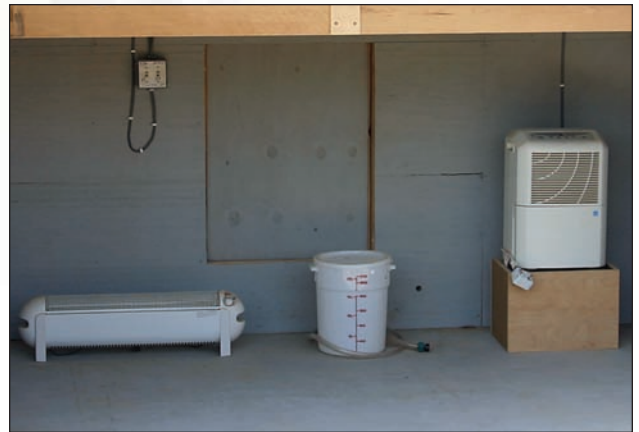
Figure 5: Heater, measuring bucket, and dehumidifier with lamp timer.
