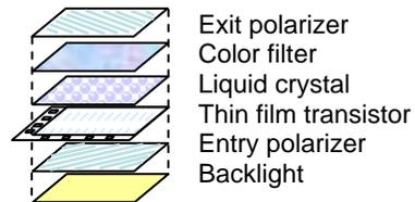
**Figure 2.** Schematic of liquid crystal display element.<sup>1</sup>
