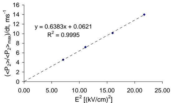
**Figure 3.** Kerr plot of the birefringence rise time in a 0.016% aqueous CNXL dispersion.
