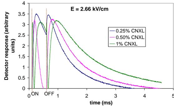
**Figure 4.** Oscillations in birefringence for various CNXL concentrations at 2.9 kV/cm
