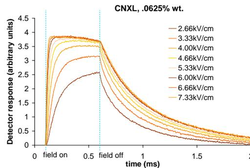
**Figure 1.** Birefringence of a 0.06% CNXL aqueous dispersion at various field strengths.
