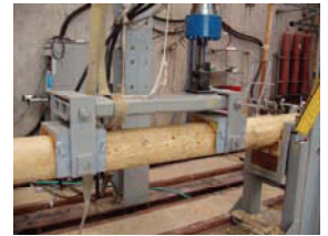
Testing the effect of through-boring on the strength of wood telephone poles.
