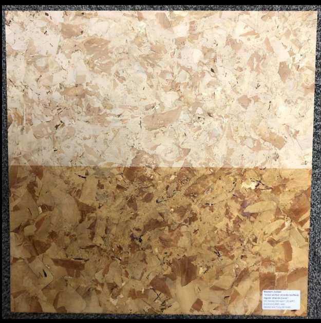
Cross-section strands (surface); regular strands (core)
