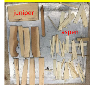
Strands produced from juniper slabs & edgings using veneer slicer
